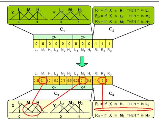
Fig. 5 Example of coding scheme considering the global LA-tuning and rule selection
